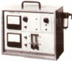
Figure 12 These analysers measure the amount of oxygen and combustibles present in flue gas.
