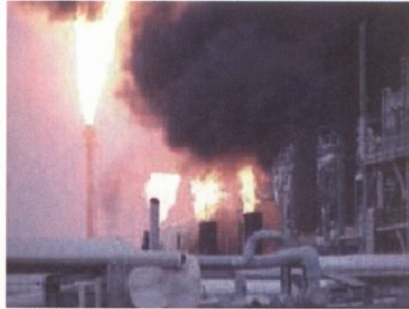
Figure 61 Flames coming out of stacks of fired heaters after tube ruptures.
