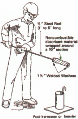
Figure 49 A regulation lighting torch. (Note: It is preferable to use a gas torch. Avoid open containers of flammables around a furnace or the operator.)
