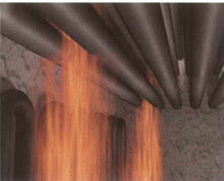
Figure 14 Flames should never strike furnace tubes, as they are shown doing in this figure.
