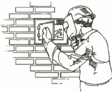
Figure 20 Use a firing shield for facial protection when looking through furnace peepholes.
